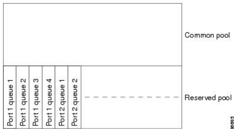
Figure 8: Egress Queue Buffer Allocation
