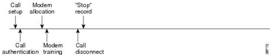
Figure 72: Modem Dial-In Call Setup Sequence With Call Disconnect Occurring Before User Authentication and With Resource Failure Stop Accounting Enabled
