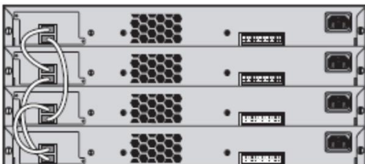
Figure 7. Four-Member Stack with 0.5-Meter Cables
