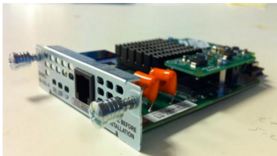
Figure 1. Single-Port EHWIC Supports VDSL2 and ADSL2/2+ for WAN Connectivity
